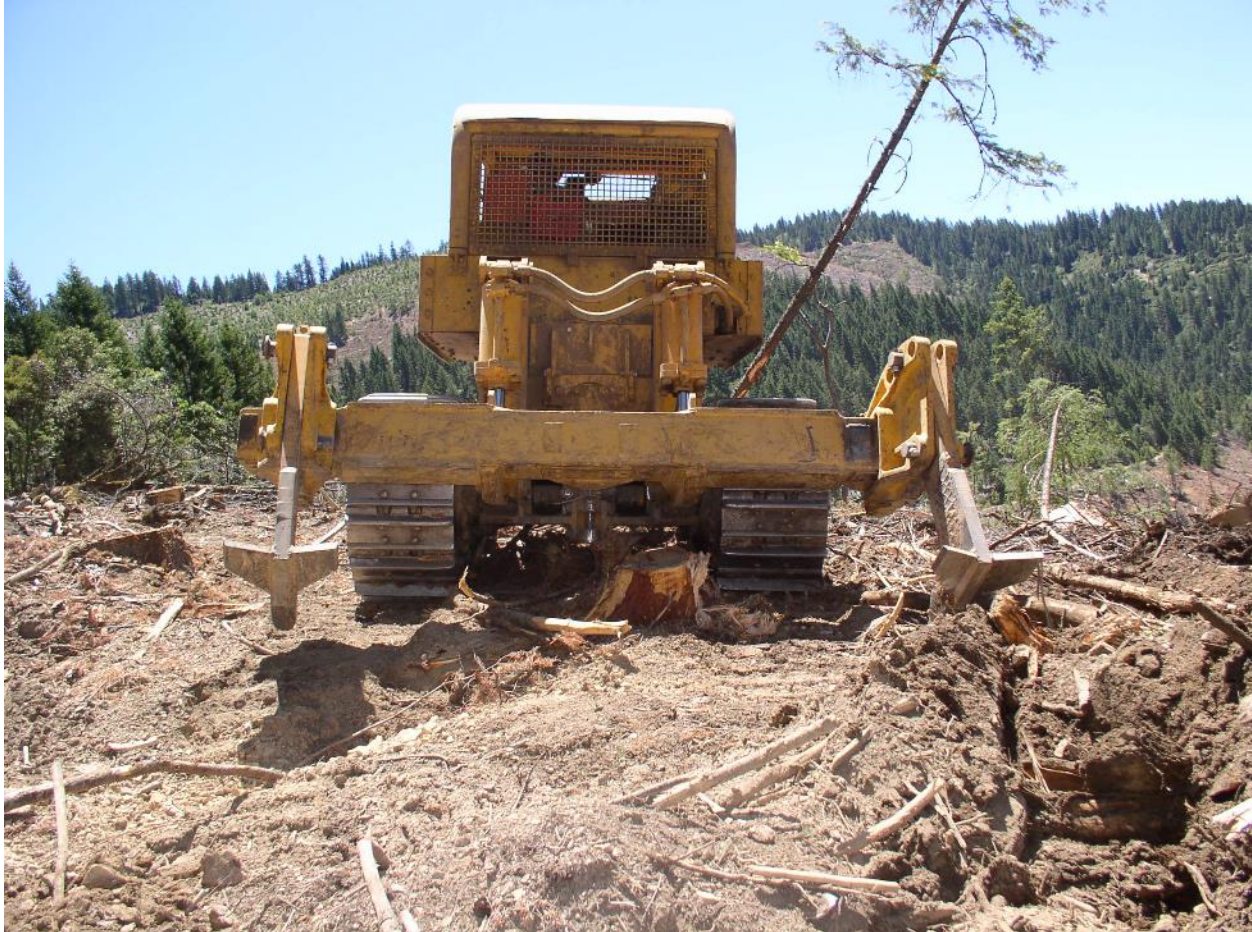
Figure 7.4 D8 with Winged Sub-soiler shanks.
