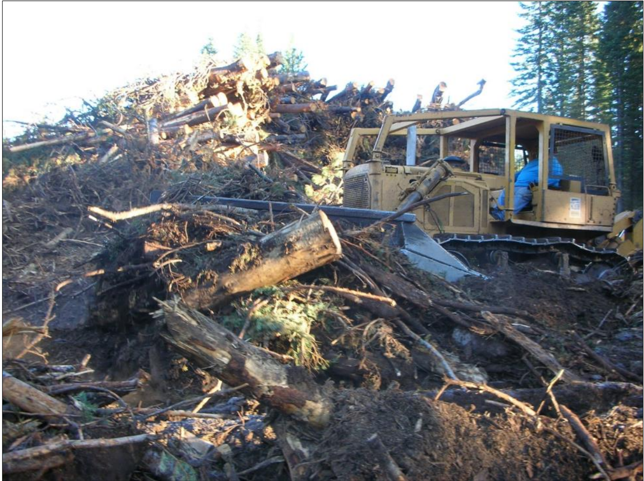
Figure 7.7 V-Blade clearing landing slash for planting.
