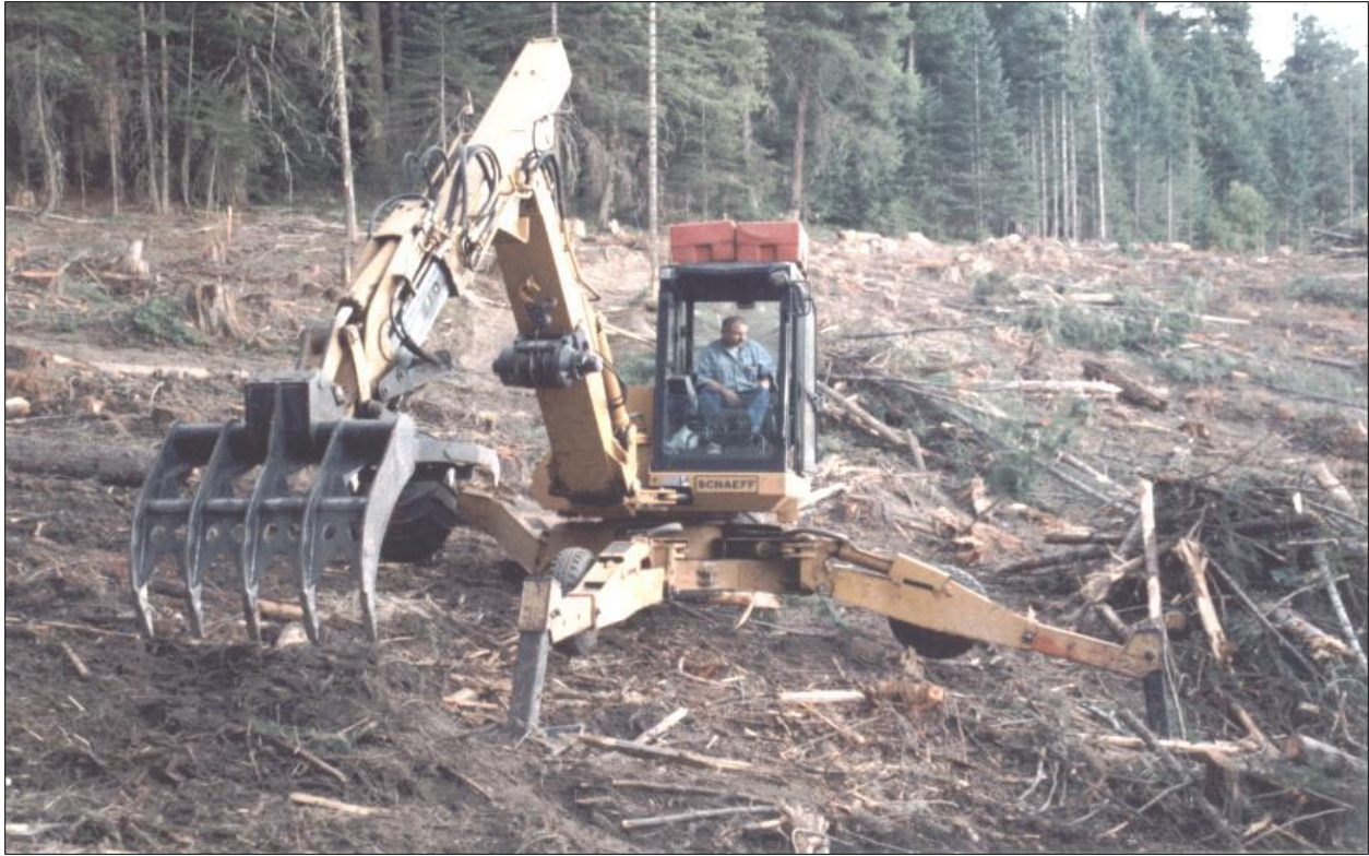
Figure 7.9 Spyder site preparation machine.
