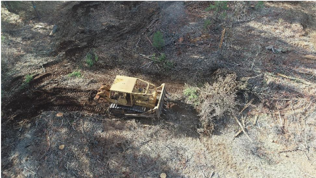
Figure 7.3 Cat with brush rake piling logging slash.
