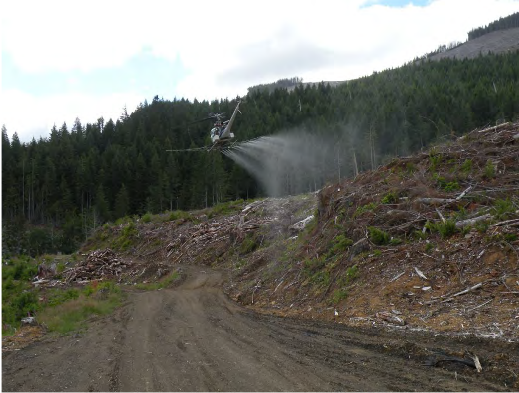
Figure 8.2 Example of a split boom application. Photo courtesy of John Mateski, Western Helicopter.
