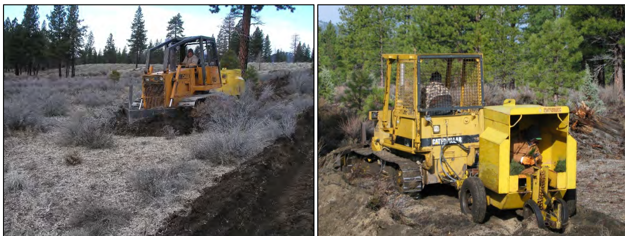
Figure 9.12 A “V Blade” attached to the front of a crawler tractor scalps away grass and brush making a level surface of moist mineral soil (left) in preparation for planting 2-0 bareroot ponderosa pine seedlings by the planting machine attached behind the crawler tractor.
